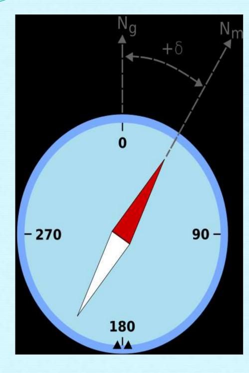
Magnetic declination, or magnetic variation, is the angle on the horizontal plane between magnetic north (the direction the north end of a compass needle points, corresponding to the direction of the Earth's magnetic field lines) and true north (the direction along a meridian towards the geographic North Pole). This angle varies depending on position on the Earth's surface and changes over time.
