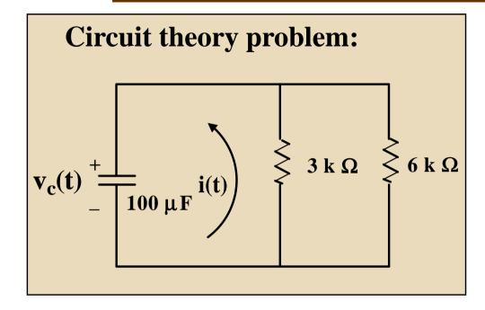
$$RC\frac{dv_{c}(t)}{dt} + v_{c}(t) = 0$$
